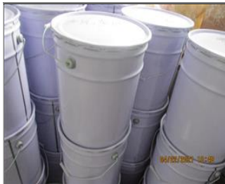
Photo of non-conformity No safety label for hazardous chemicals.JPG
